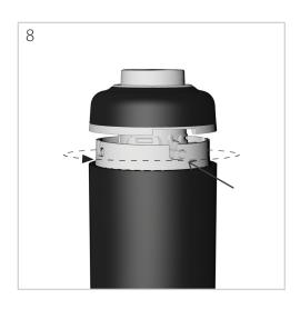
To reassemble, ensure that the O-ring is seated in the groove at the bottom of the end cap, align the pins on the end-cap, and push downwards, and twist slightly counter-clockwise until the pins return to the locked position. Finally, replace the retaining clip by firmly pressing straight down until it "clicks" into place.
