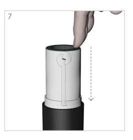
Insert the rolled inner foam baffling material into the body of the Qtube and push all the way until the bottom of the material contacts the opposite end of the Qtube body. You should be able to look down the center of the material and see that the center is clear and that there are no obstructions to the airflow.
