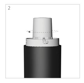
Grasp the top of the End Cap and twist slightly clockwise until the pins line up with the vertical slots on the body of the Qtube.
